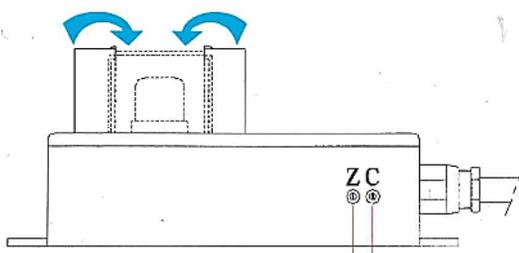
The gas to analyze is picked up by diffusion through a metal gate.
